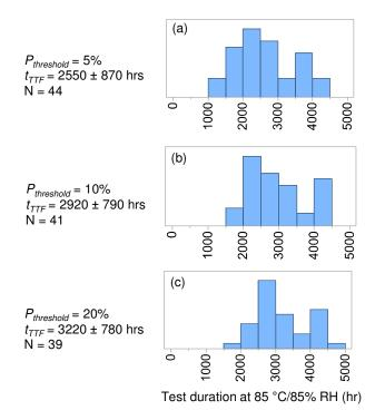
Figure 4: Histograms representing the time-to-failure in hours at 85 °C/85% RH corresponding to 5%, 10% and 20% module Pmax loss. Mean, standard deviation and module count is compiled for each time-to-failure threshold.
