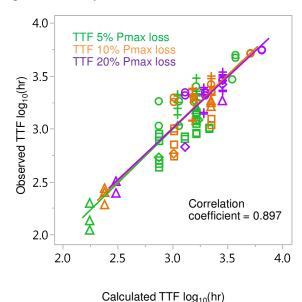
Figure 1: Observed and calculated time-to-failure (TTF) data under damp heat conditions for c-Si solar cells in a glass-polymer package with EVA encapsulant. The marker shape represents the data source as follows:  $\Diamond$  [7], + [8],  $\Delta$  [9],  $\bigcirc$  [10],  $\Box$  this paper. The time to failure data is fit to the power law relation,  $t_{TTF} = A * e^{\wedge}(E_a/kT) * RH^{\wedge}(n)$ , where  $E_a = 0.89$  eV, and n = -2.2.
