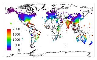
Figure 2. Global map of acceleration factors, with a color scale to represent the test duration in hours at 85 °C/85% RH that is expected to correspond to 25 years of operation in the field. Each data point represents a TMY data set that is interpreted using the stress model (1).
