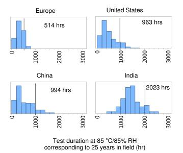
Fig. 3: Histograms representing the test duration in hours at 85 °C/85% RH that is expected to correspond to 25 years of operation in the field. The vertical lines designate the location at the 90<sup>th</sup> percentile stress amount.
