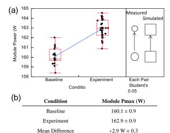
Fig. 5. Module power results from the comparison of baseline and experimental cell interconnect designs. Experimental cell interconnect design shows +2.9 W (+1.8% relative) mean module power improvement.
