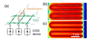
Fig. 1. (a) schematic of the distributed-element circuit analysis approach for optimizing metallization and TCO design. (b) Measured and (c) simulated electro-luminescence images from a solar cell of interest.
