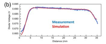
Fig. 2. Electroluminescence (EL) line scan overlays based on the images from Fig. 1b and 1c. Both (a) vertical and (b) horizontal EL line scans show the close correspondence between measurement and simulations.
