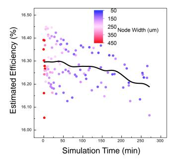
Fig. 6. Scatter plot showing estimated device efficiency results for a range of simulation node width values. The standard deviation in estimated device efficiency is found to decrease with smaller node size. Simulations with node width values  $<200~\mu m$  were found to provide efficiency estimates with a standard deviation value <0.05% abs.
